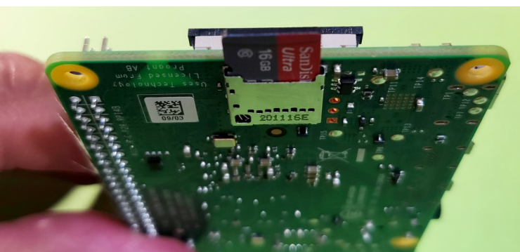
Raspberry Pi 4 Model B Micro SD Slot
